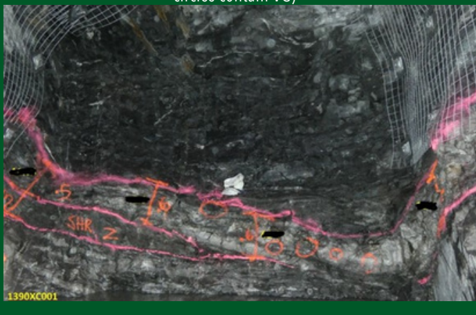
View East, 1390mRL Penny North Main Vein - Hanging Wall (painted circles contain VG)
