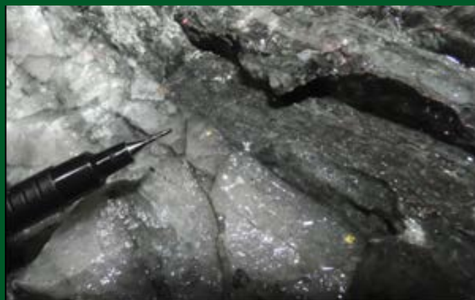
Fine Visible Gold within HW Penny North Main Vein
